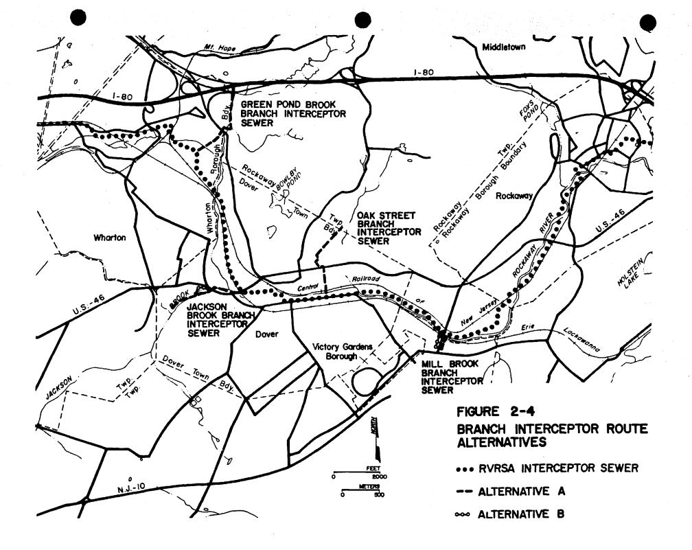
Because the Oak Street Branch Interceptor uses an existing ROW, no alternative alignment is necessary. This branch interceptor is intended to relieve the overloaded local collection system in Dover (Killam, 1978). These feasible alternatives will be discussed further in this chapter.
